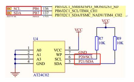
Figure 9 Diagram of Connection between APM32F103ZE and AT24C02
