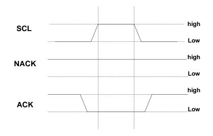
Figure 7 ACK and NACK Signal Timing Diagram
