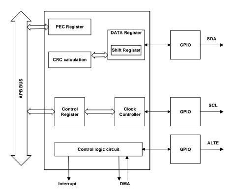
Figure 1 I2C Function Structure Diagram
